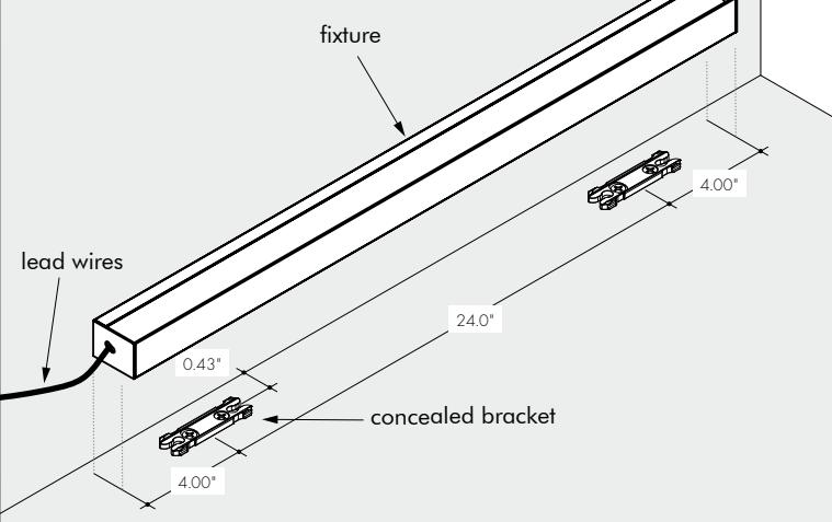
**1.1** Determine the location of where the fixture(s) will be installed. Lay the fixture(s) on the surface, and make any necessary reference marks for the concealed bracket. Make marks 4" from each end of the fixture(s) and also every 24" in between. Use the fixture profile and mounting bracket detail, for any additional details.
