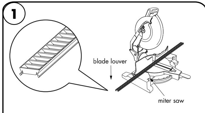
**1.1** Use miter saw to cut the blade louver into desired length. Make sure blade louver and fixture lens are the same length.
