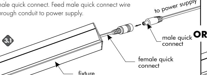
**Option 2** Feed wire leads to the power supply.
