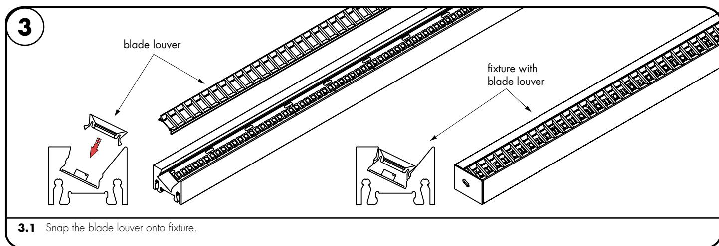
**3.1** Snap the blade louver onto fixture.
