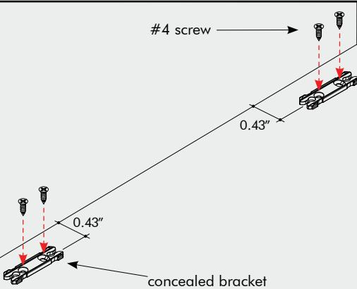
**2.1** Align the mounting brackets to the marks, followed by securing each mounting bracket with 2 screws. Snap the extrusion into the mounting brackets.
