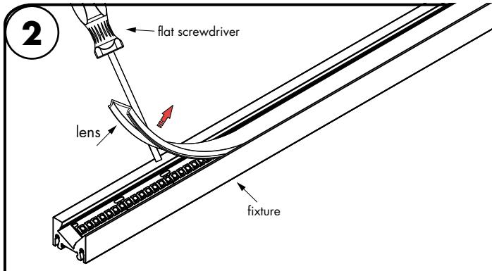
**2.1** Use a flat screwdriver to remove the fixture lens.
