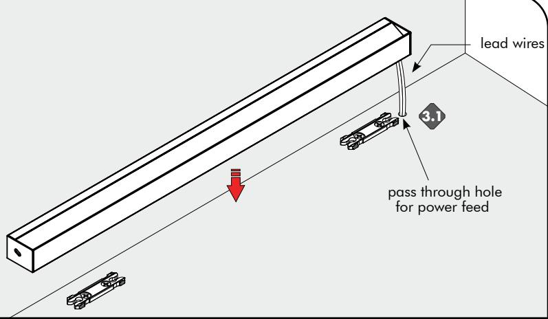
**3.1** If necessary make any pass through holes for wire lead/connector to the surface, depending on the power feed option. Then snap the fixture into the concealed mounting bracket to secure in place.
