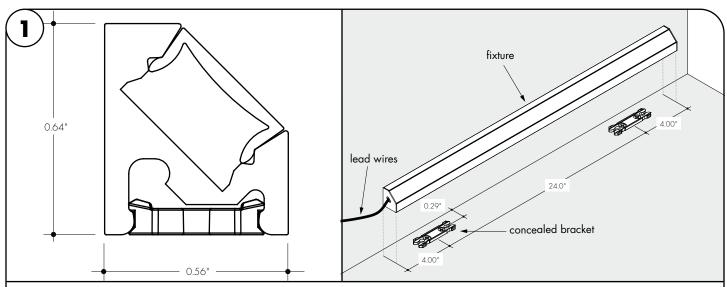
1.1 Determine the location of where the fixture(s) will be installed. Lay the fixture(s) on the surface, and make any necessary reference marks for the concealed bracket.
