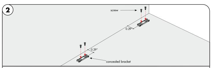
2.1 Align the mounting brackets to the marks, followed by securing each mounting bracket with 2 screws. Snap the extrusion into the mounting brackets.
