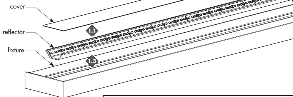
**1.1** From the inside of the fixture, carefully insert a flathead screwdriver to the edge. Followed by carefully pulling on the cover to remove.
