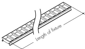
This Black louver/lens combo comes in 12" increments and sits in place of a Myka lens, not in addition to.
