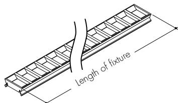
This White louver/lens combo comes in 12" increments and sits in place of a Myka lens, not in addition to.
