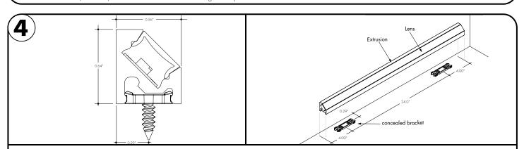
**4.1** Align the mounting brackets to the edge of the surface, followed by securing each mounting bracket with 2 screws. Mounting bracket must be installed every 24". Snap the extrusion into the mounting brackets. Reference dimensions for additional details.
