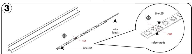
3.1 LineLED can be shortened by cutting along the dashed lines in between the solder pads. Make sure the cut is made on the side of the LineLED without the wire leads. LineLED cannot touch the metal endcap which will shorten the circuit.
