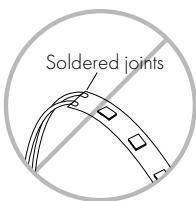
NOTE - Avoid bending near 1" on both side of the soldered joints.
