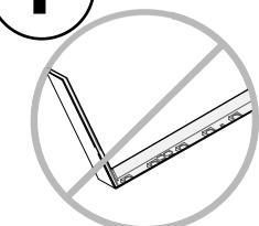
NOTE: Avoid bending the lineLED in sharp horizontal angles, doing so can cause damage to the LEDs.
