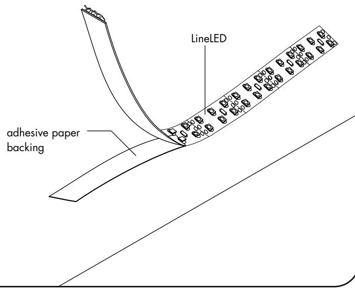
NOTE - When removing backing & laying LineLED to surface avoid installing with ripples & bending over 90°.
