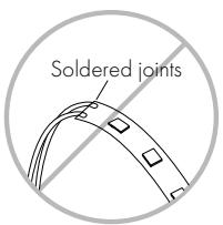
NOTE - Avoid bending near 1" on both side of the soldered joints.
