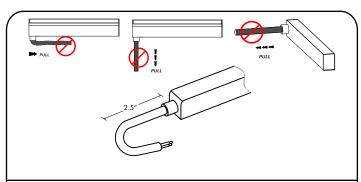
Do not pull the cable, otherwise it may disable the function of the connector and lead to water ingression. It's recommended to keep the first 2.5 inches of the cable straight and without tension.
