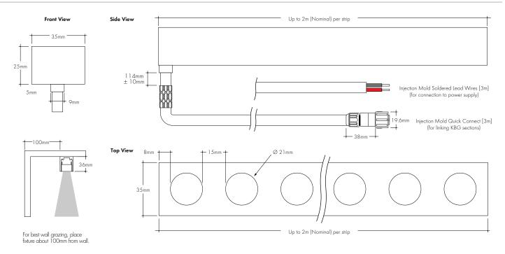
Note: Each 2m Kurba Grazer 3D<sup>TM</sup> section is 48W. Two 2m Kurba Grazer 3D<sup>TM</sup> strips may be joined together in series up to 4m for a continuous run.
