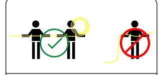
When light length longer than 6ft, make sure somebody helps to lift the light, in case the heavy weight of light itself generates too small bending angle or twisting, which may damage Kurba.
