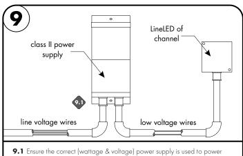
LineLED. Then proceed to connect LineLED wires from channel to power supply. For more information please refer to power supply and LineLED wiring instructions.
