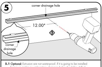
facing up and in a wet location, drainage holes should be drilled along the inner corner of the channel every 12". Drill 1/16" to 1/8" diameters holes before installing LED strip.
