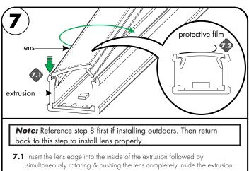
7.2 Remove the protective film from the diffuser lens.
