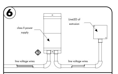
6.1 Ensure the correct (wattage & voltage) power supply is used to power LineLED. Then proceed to connect LineLED wires from extrusion to power supply. For more information please refer to power supply and LineLED wiring instructions.
