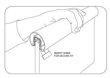
13 If using handrail with glass, insert handrail with completed cap rail housing and LED light engine onto glass once all the above steps are completed. Glass enters base of cap rail housing and stops at interior housing tabs. Note: If loose after glass insertion, cut LED housing shims to size and insert between glass and housing.
