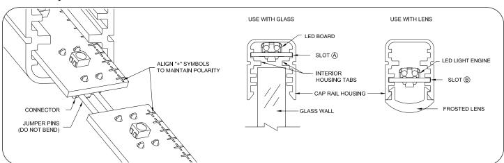
3 Slide LED light engine boards into cap rail housing slot. If using with glass, place LED light engine board into slot (A). Slot options (A) or (B) are available if using with lens. Once inserted, take two jumper pins and insert into female connectors on end of LED light engine board light. To connect LED boards, align the "+++" of the first board to the "+++" on the second LED board. Press the two tabs on the connector to remove jumper pins and lead wires.
