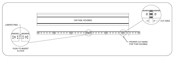
4 Slide LED light board into the extended jumper pins until boards link securely together. Custom cut option is described in Step 5.
