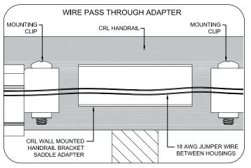
10 The CRL Saddle Adapter is designed to allow LED wiring to pass through inside of handrail and should be used where needed.
