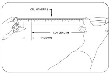
1 Measure the distance between handrail supports. Subtract 2" (51mm) total from the measurement to allow for clip space.
