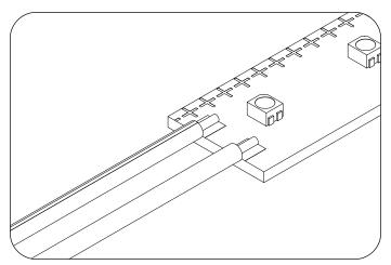
6 If the cut piece is in middle of run, prepare LED light engine board by using a soldering iron tip with solder to burn off transparent waterproof coating at LED light board cut lines. Then solder 18 AWG jumper wires to cut LED board to connect to adjacent LED board. Note: The black & white striped wire is positive (+) and black wire is negative (-).
