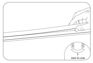
12 Gently snap on lens at end of cap rail housing. Continue to press lens down length of housing channel, snapping it securely in place.
