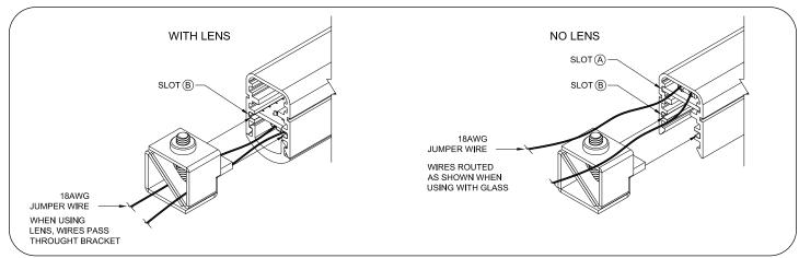
7 If using lens, feed 18 AWG jumper wire through LED mounting clip as shown (above left), and slide clip in cap rail into Slot B.
