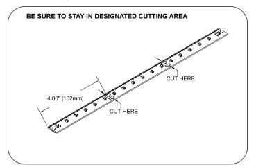
5 The LED light engine board is designed to be cut in 4" (102mm) lengths as indicated by the double lines on the LED board. Use a hack saw or other fine toothed saw to cut the LED board. If cut LED board is used at the end of run, no soldering is required. Note: the remainder LED light engine board is usable elsewhere if needed.
