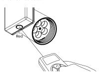
To complete the process, hold the button and aim the laser away from the sensor. The LED on the spotlight will flash green to indicate that the Start Address has been received.
