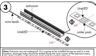
Note: Extrusion are not waterproof. If it is going to be installed facing up and in a wet location, drainage holes should be drilled along the inner corner of the extrusion every 12". Drill 1/16" to 1/8" diameters holes before installing LED strip
