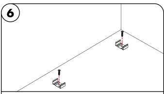
6.1 Use #4 screw to screw mounting brackets into previously made markings from step 1, then clip the extrusion on to the mounting brackets. Mounting Mounting bracket must be installed every 15"
