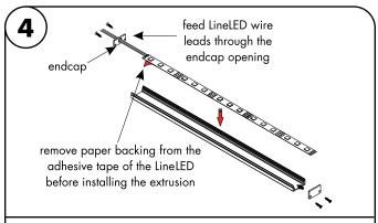
Prior to installing LineLED to extrusion, clean extrusion from any debris. Gently push LineLED onto aluminum extrusion. Then install endcaps at each ends of the extrusion
