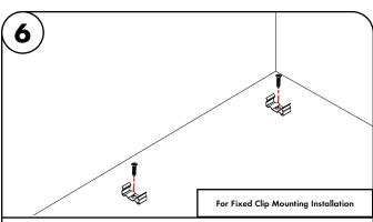
Use #4 screw to screw mounting brackets into previously made markings from step 1, then clip the extrusion on to the mounting brackets. Mounting Mounting bracket must be installed every  $15^{\prime\prime}$
