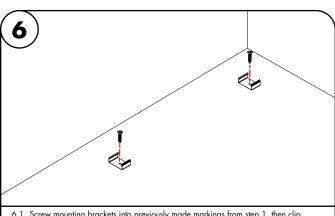
Screw mounting brackets into previously made markings from step 1, then clip the extrusion on to the mounting brackets. Mounting bracket should be installed every 15"
