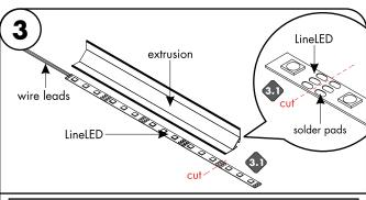
Note: Extrusion are not waterproof. If it is going to be installed facing up and in a wet location, drainage holes should be drilled along the inner corner of the extrusion every 12". Drill 1/16" to 1/8" diameters holes before installing LED strip
