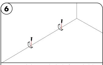
Screw mounting brackets into previously made markings from step 1, then clip the extrusion on to the mounting brackets. Mounting bracket should be installed every  $15^{\prime\prime}$
