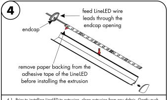
Prior to installing LineLED to extrusion, clean extrusion from any debris. Gently push LineLED onto aluminum extrusion. Then install endcaps at each ends of the extrusion.
