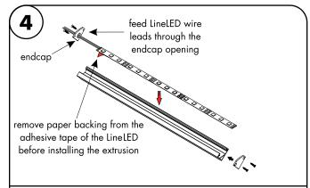
4.1 Prior to installing LineLED to extrusion, clean extrusion from any debris. Gently push LineLED onto aluminum extrusion. Then install endcaps at each ends of the extrusion.
