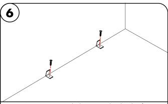
6.1 Use #4 screw to screw mounting brackets into previously made markings from step 1, then clip the extrusion on to the mounting brackets. Mounting bracket must be installed every 15"
