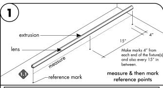
**Note:** Complete fixture must be built prior to installing. To make all necessary reference marks & to also ensure all parts are included. Then it can be taken apart for installation.
