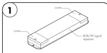
Remove covers on both sides of RGBW signal repeater by using a small phillips screwdriver. Store covers and their fasteners until repeater setup is complete and functioning properly and then re-install them.
