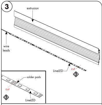
3.1 LineLED can be shortened by cutting along the dashed lines in between the solder pads. Make sure the cut is made on the side of the LineLED without the wire leads. LineLED cannot touch the metal endcap which will shorten the circuit.
