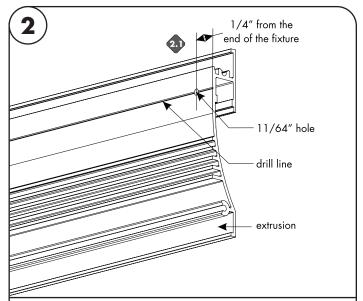
2.1 Remove the lens from the inside of the extrusion, and from one end of the extrusion. Make a 11/64" hole on the drill line from 1/4" end of the extrusion for wire management.
