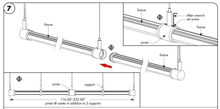
If joining fixtures together, insert the fixture end into the corresponding fixture. Secure by tightening the two set screw that is the closest to the fixture. Reference drawing above as reference, to join correctly.
