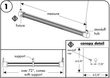
Note: Prior to installation all 24VDC wires must be present in junction box. Refer to the power supply installation instruction for additional information.
