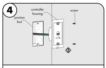
4.1 Align the controller housing to the junction box and secure using the two screws.
