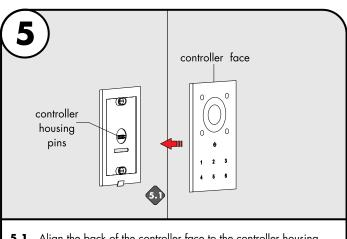
**5.1** Align the back of the controller face to the controller housing pins and snap in to secure.
