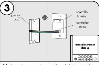
Loosen the screws on the back of the controller housing and make all the proper wiring and then re-tighten screws. Refer to the wiring diagram on page 2 for additional information.
