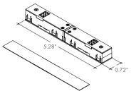
For electrically joining adjacent Track sections
