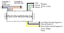
WARM DIM CURVE (WITH TUNABLE WHITE MODULE), 0-10V WITH LUTRON ATHENA, 0.1%, PS-010V-WD-D-96-24-AWNR
