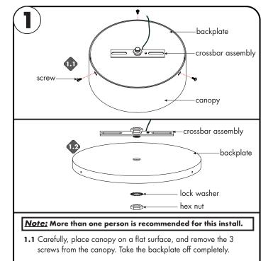
1.2 Remove the crossbar assembly from the backplate.
