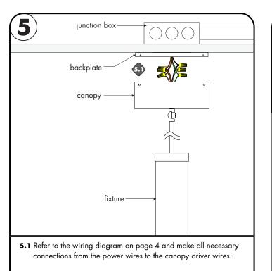
5.2 Connect to ground in accordance with local electrical codes.
