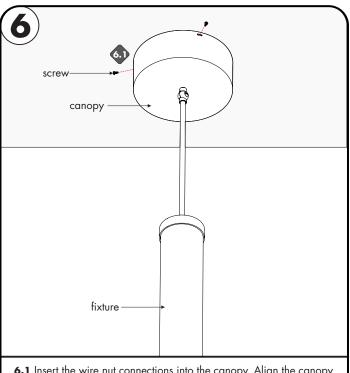
**6.1** Insert the wire nut connections into the canopy. Align the canopy to the backplate and securing using the 3 screws.
