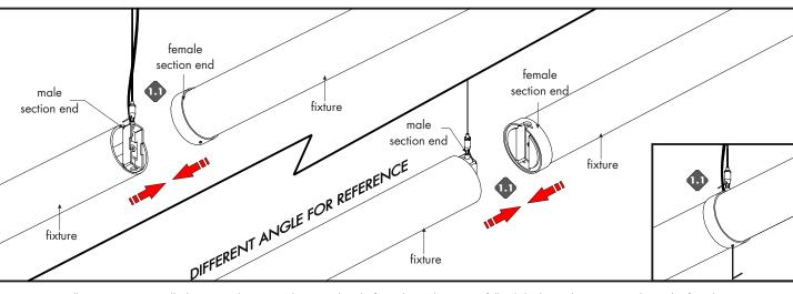
1.1 Once all sections are installed & set to the proper hanging height from the ceiling. Carefully slide the male section end into the female section end, and secure be tightening the set screws on the top & bottom of the female section end. Repeat for any other sections that need to be joined.
