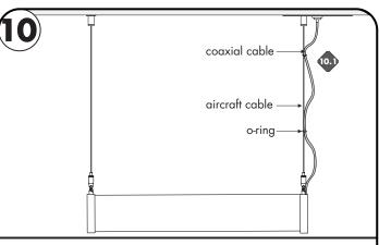
**10.1** If necessary make any final adjustments to the cables use the o-rings for a cleaner look.
