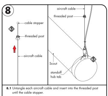
8.2 Push on the standoff hub tab and feed the aircraft cable into the standoff hub until necessary. Release tab to secure in place. For
