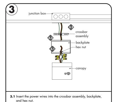
3.2 Refer to the wiring diagram on page 6 and make all necessary connections from the power wires to the canopy driver wires.
