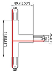
T FEED FOR 2 CIRCUIT APPLICATION - TYPE C
