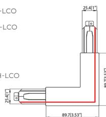
**T FEED FOR 2 CIRCUIT APPLICATION - TYPE A**
