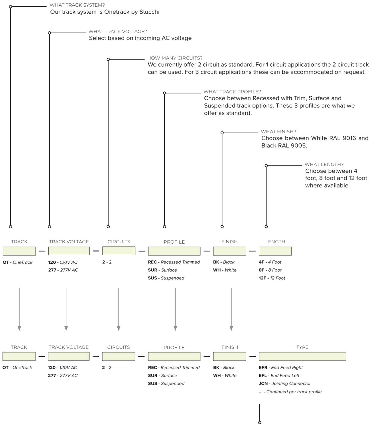
Ensure that your selection of Track, Voltage, Circuits, Profile and Finish matches between the Track and Accessories.
