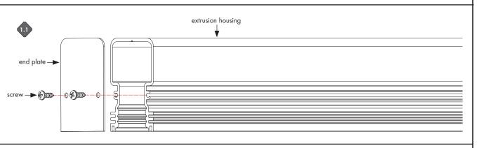
1.1 Screw end plate onto extrusion housing.
