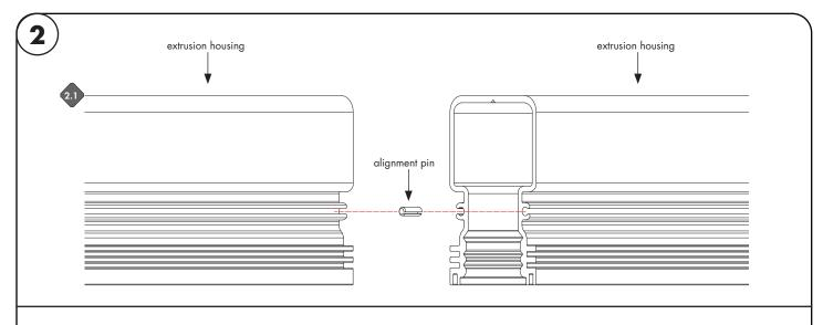
**2.1** If more than one extrusion housing, use two alignment pins to connect both side of the extrusion housing.
