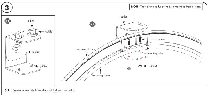
3.2 Connect collar with mounting frame by screws. Use locknut to secure collar.
