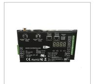
DMX512 decoder with RDM functionality features 5 PWM output channels with common anode. High PWM output frequency range allows the product to be used in HD video conferencing spaces.
