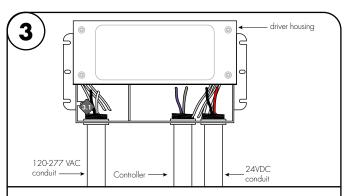
**3.1** Insert the 120-277 VAC power into the driver housing from the electrical panel. Followed by bringing the 24V DC low voltage wires from the LEDs into the driver housing. In addition bring the controller wire if applicable. Refer to diagram on page 2 to make all the proper wiring connecitons.
