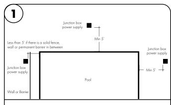
1.2 Power supply must be placed 5 feet horizontally away from the inside walls of the pool unless separated from the pool by a solid fence, wall, or other permanent barrier.
