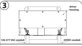
3.1 Insert the 120-277 VAC power into the driver housing from the electrical panel. Followed by bringing the 24V DC low voltage wires from the LEDs into the driver housing. In addition bring the controller wire if applicable. Refer to diagram on page 2 to make all the proper wiring connections.
