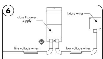
**6.1** Ensure the correct (wattage & voltage) power supply is used to power the fixture. Then proceed to connect the fixture wires from fixture to the power supply. For more information please refer to power supply wiring instructions.
