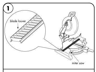
1.1 Use miter saw to cut the blade louver into desired length. Make sure blade louver and fixture lens are the same length.
