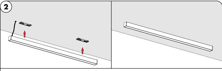
2.1 If necessary make any pass through holes for wire lead/connector to the surface, depending on the power feed option. Then snap the fixture into the concealed bracket to secure in place.
