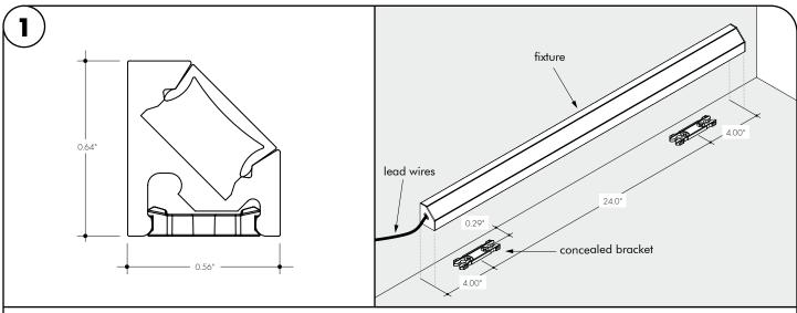
1.1 Determine the location of where the fixture(s) will be installed. Lay the fixture(s) on the surface, and make any necessary reference marks for the concealed bracket. Make marks 4" from each end of the fixture(s) and also every 24" in between. Use the fixture profile and mounting bracket detail, for any additional details.
