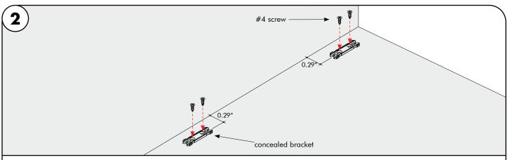
Align the mounting brackets to the marks, followed by securing each mounting bracket with 2 screws. Snap the extrusion into the mounting brackets.
