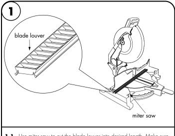
1.1 Use miter saw to cut the blade louver into desired length. Make sure blade louver and fixture lens are the same length.
