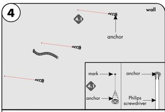
Align the anchors onto the marks and tap until the threaded section. Then screw in the threaded portion of the anchors with a Philips screw driver.
