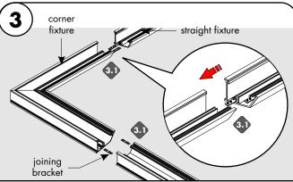
3.1 IF CONNECTING MULTIPLE FIXTURES TOGETHER: Insert the joining brackets into one of the fixture end(s) & tighten the screws on the bracket. Then slide the connecting fixture into the brackets and secure by tightening the screws on bracket.
