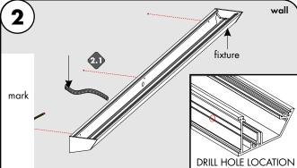
Prior to installing the fixture, power wires must be present near fixture. Lay the fixture on the desired location, & mark the mounting holes to the wall. If fixture center hole doesn't match up with the conduit. Make an additional 1/2" hole to the back of the extrusion. Use diagram above to make hole in the correct location.
