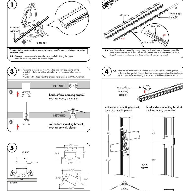
5.1 1 If necessary route slots on surface with the proper width and depth to accommodate aluminum extrusion (reference step 7 for slot width).
