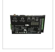
DMX512 decoder with RDM functionality features 5 PWM output channels with common anode. High PWM output frequency range allows the product to be used in HD video conferencing spaces.
