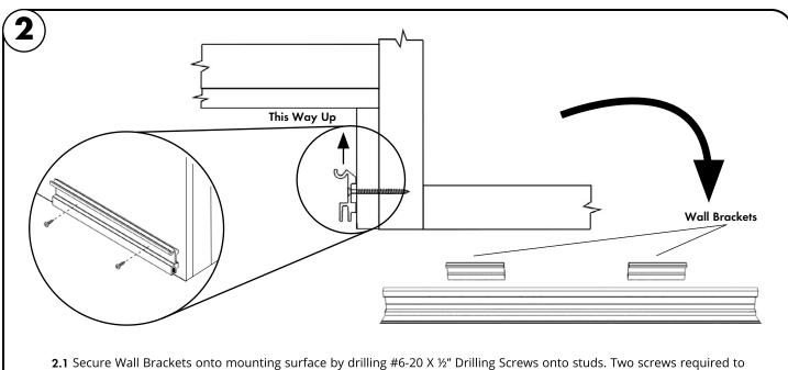
mount each Wall Bracket. Wall Bracket can be field cut to accommodate length of Blade Body.
