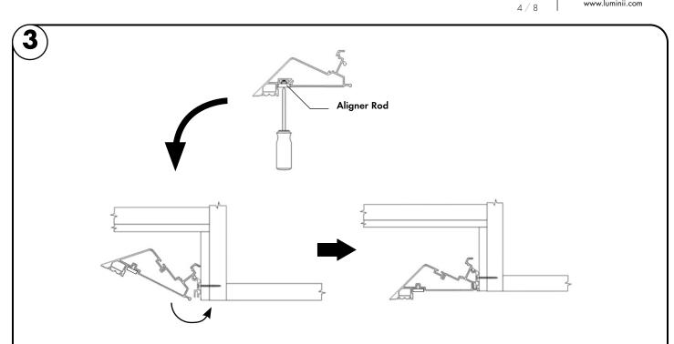
3.1 Insert Aligner Rods into Aligner Rod slot at the bottom of the Blade Body to be used later to join multiple runs/corners together.
