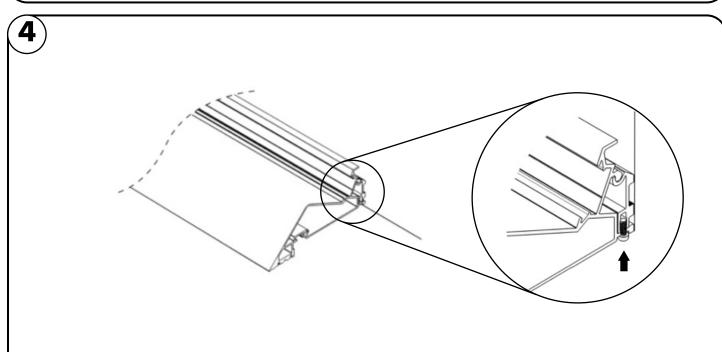
**4.1** Lock the Blade Body to the Mounting Bracket using Locking Screw.
