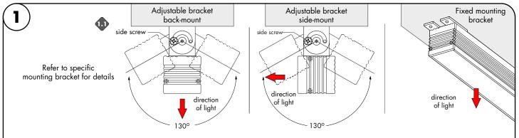
**1.1** Determine the location of the install. Use the pre-installed mounting bracket holes as a guide, then mark the desired location. If using adjustable mounting brackets, side screws must be loosen to rotate.
