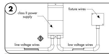
Ensure the correct (wattage & voltage) power supply is used to power the fixture. Then proceed to connect the fixture wires from fixture to the power supply. For more information please refer to power supply wiring instructions.
