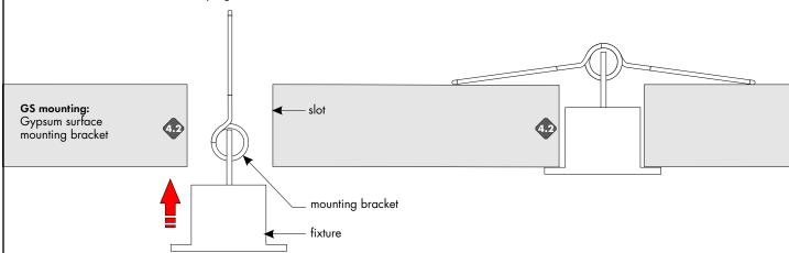
4.3 For no surface mounting bracket option: Apply construction adhesive to the bottom of the cutout slot, then place fixture onto adhesive to secure
