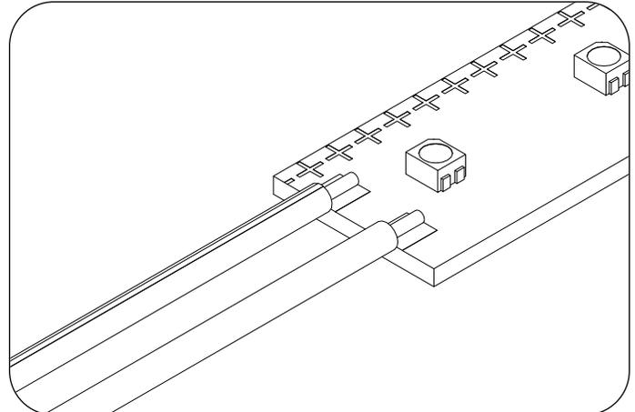
**6** If the cut piece is in middle of run, prepare LED light engine board by using a soldering iron tip with solder to burn off transparent waterproof coating at LED light board cut lines. Then solder 18 AWG jumper wires to cut LED board to connect to adjacent LED board. Note: The black & white striped wire is positive (+) and black wire is negative (-).
