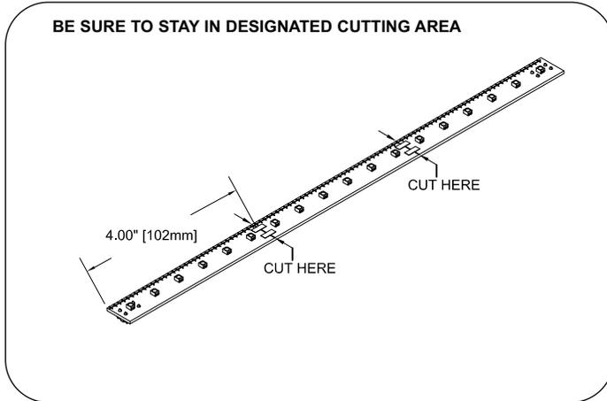
**5** The LED light engine board is designed to be cut in 4" (102mm) lengths as indicated by the double lines on the LED board. Use a hack saw or other fine toothed saw to cut the LED board. If cut LED board is used at the end of run, no soldering is required. Note: the remainder LED light engine board is usable elsewhere if needed.
