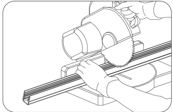
**2** Take reduced measurements and cut cap rail housing to length with chop saw. If using lens, cut lens to same length as cap rail housing. Do not cut both at same time.
