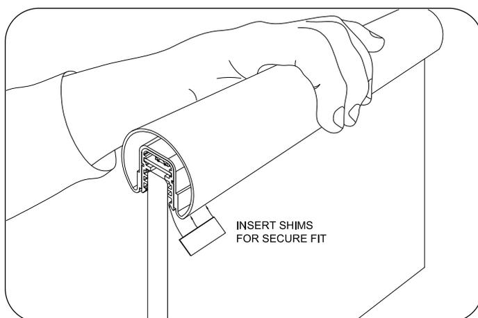
**13** If using handrail with glass, insert handrail with completed cap rail housing and LED light engine onto glass once all the above steps are completed. Glass enters base of cap rail housing and stops at interior housing tabs. Note: If loose after glass insertion, cut LED housing shims to size and insert between glass and housing.
