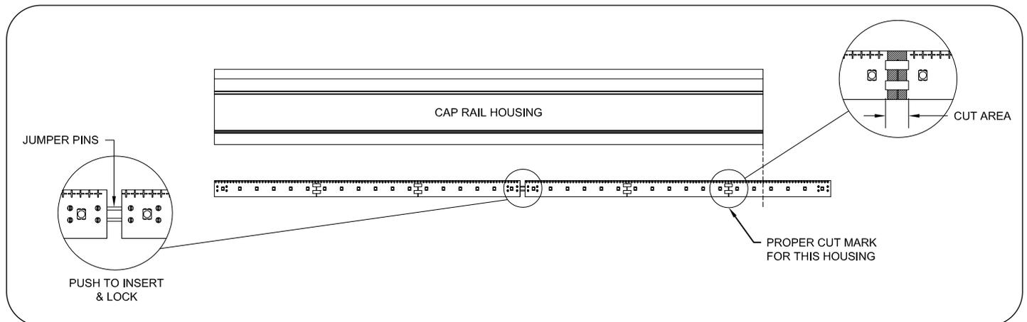
**4** Slide LED light board into the extended jumper pins until boards link securely together. Custom cut option is described in **Step 5**.
