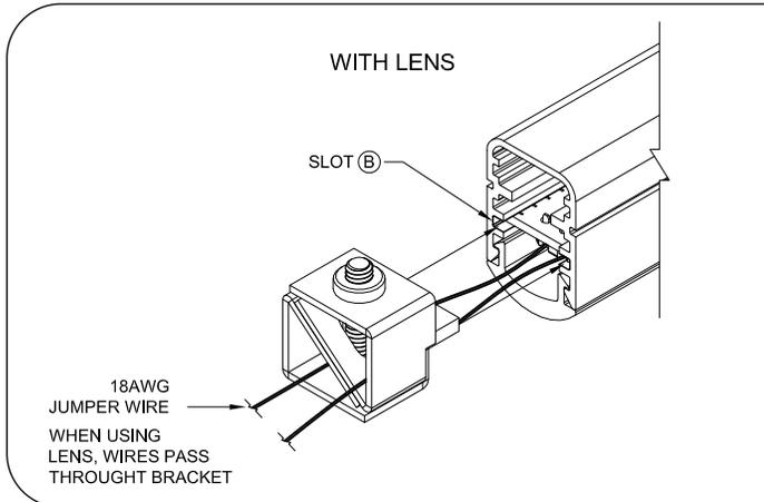
**7** If using lens, feed 18 AWG jumper wire through LED mounting clip as shown (above left), and slide clip in cap rail into Slot (B).
