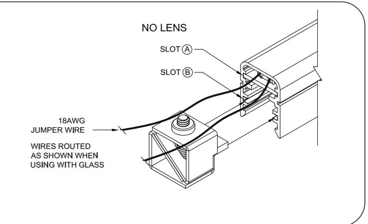
**8** If lens is not used, feed 18 AWG jumper wire as shown (above right), and slide clip in cap rail housing into Slot (B).
