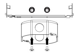
Examine your joist material. If the joist is wood, hammer in nail support (if applicable) and fix the construction bracket in position with wood screws or nails. If the joist is metal, use suitable screws.
