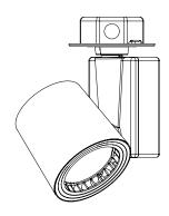
The junction box required for installation should not exceed 4" in diameter and requires 2x #8-32 UNC threaded mounting holes positioned 3 ½" (89mm) apart from the centre of origin.
