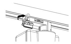
Rotate tab (D) to the desired circuit position (see
