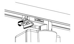
With the 2-Circuit track adaptor, you can choose which circuit the luminaire is connected to:
