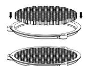
Insert the accessory holder up through the DRX7 face plate and magentically attach to the optic holder.
