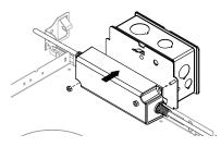
$\label{eq:power_supply_flying} 2 \quad \text{Feed the power supply flying lead into the junction box} \\ \text{via the hole provided.}$
