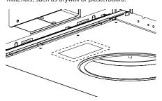
DRX7 is rated for use in insulated ceilings with zero clearance to building members.
