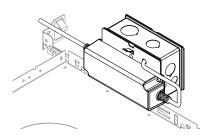
Bring field wiring in through the provided knockouts in the junction box.
