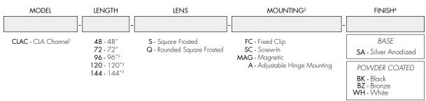
End Caps are included with channel, one of H3 (no hole) and one of H4 (with hole). Order additional End Caps as necessary. Mounting Clips are included with channel. Refer to chart above for provided mounting clip quantities. Order additional Mounting Clips as necessary.
