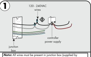
controller housing 900000 tab contractor) to connect controller properly. 2.1 Carefully insert a flat screw driver into the controller housing tab 1.1 Connect the white (neutral) & black (hot) power supply wires to and slightly pull up until controller face comes off. the white & black power wires (120 - 240VAC).
