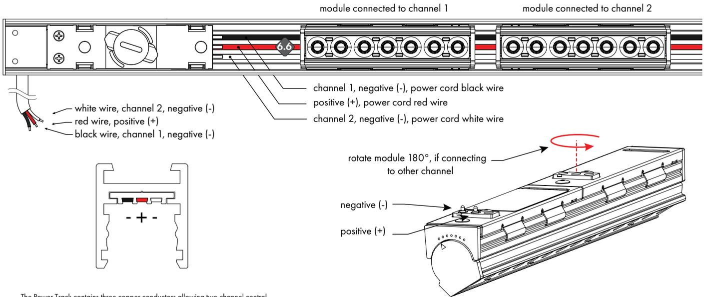
The Power Track contains three copper conductors allowing two channel control .
