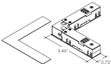
For use with Mechanical L Joiner
