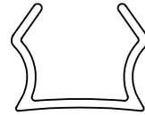
Track Covers ship complete with Recessed Trimless Track and cover unoccupied sections of track. They are field cuttable and can be used to protect channel during the mudding process. Additional can be ordered, if necessary.
