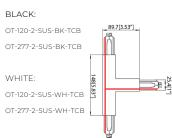
T FEED FOR 2 CIRCUIT APPLICATION Compatible with all tracks
