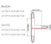
T FEED FOR 2 CIRCUIT APPLICATION - TYPE C Compatible with all tracks
