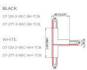
T FEED FOR 2 CIRCUIT APPLICATION - TYPE C To be used with recessed cover, codes below for assembled unit
